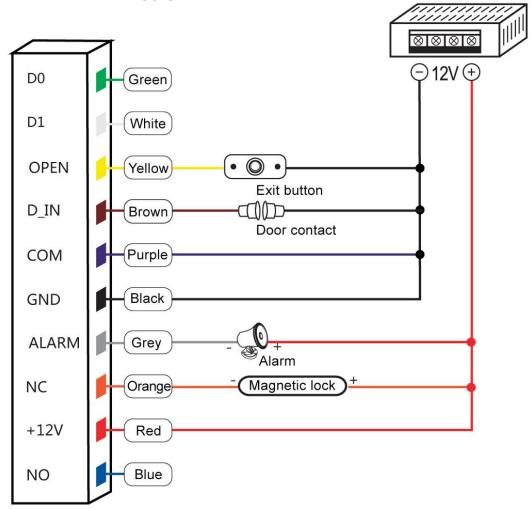
Note: The door contact and alarm function are optional
